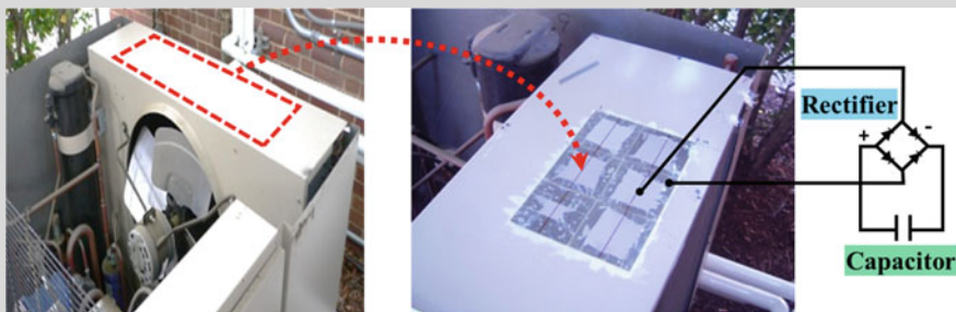
Fig. 8.12 Piezoelectric energy harvesting skin for powering wireless sensors
